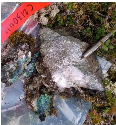
#C2130416 : 13.70% Cu, 4.83 g/t Au, 28.60 g/t Ag Clusters of digenite and malachite in a quartz and calcite vein within a mafic host rock heavily altered with epidote and albite
