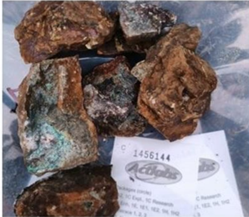
C1456144 : 0.54% Cu, 41 ppm Co Epidotized gabbro outcrop containing 7% malachite and 3% chalcopryrite
