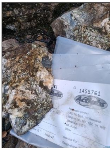
C1455761 : 6.12% Cu, 280 ppb Au, 1.77% REE, 675 ppm Co, 6.80 g/t Ag
