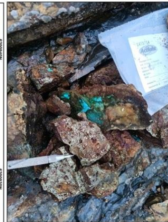
C1455754 : 27.60% Cu, 877 ppb Au, 0.06% REE, 3450 ppm Co, 32.40 g/t Ag
