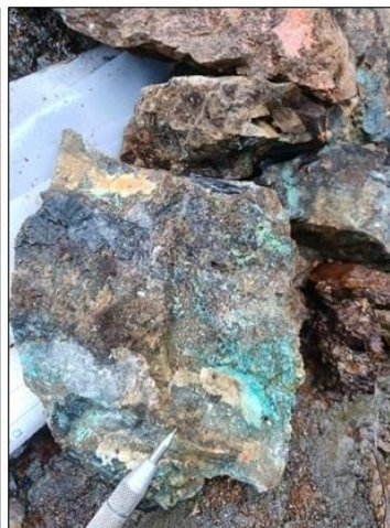
C1455755 : 2.53% Cu, 136 ppb Au, 0.87% REE, 168 ppm Co, 3.10 g/t Ag
