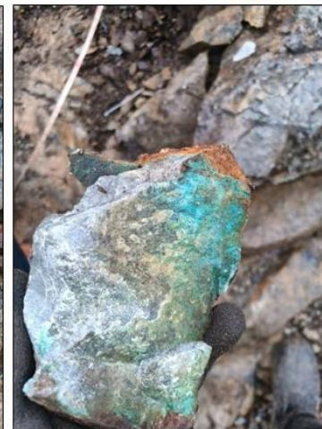
C1455757 : 4.59% Cu, 61 ppb Au, 0.58% REE, 125 ppm Co, 2.60 g/t Ag
