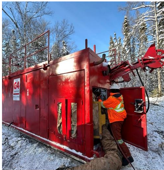
Installation of the Drill Rig at Site 2026-1, Hole FL-26-287.
