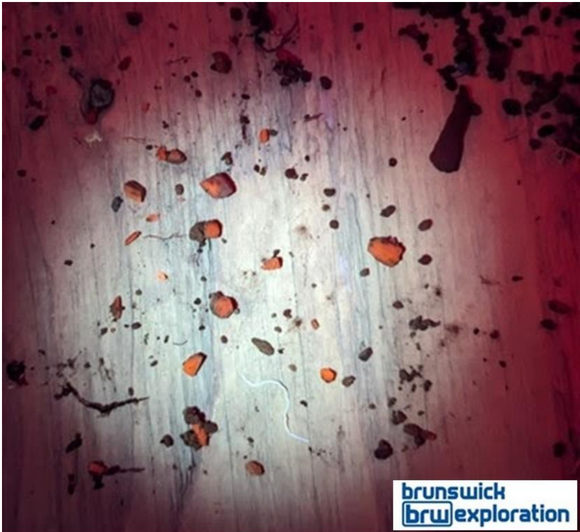
Photo of orange-fluorescent spodumene grains in till lighted by UV lamp
