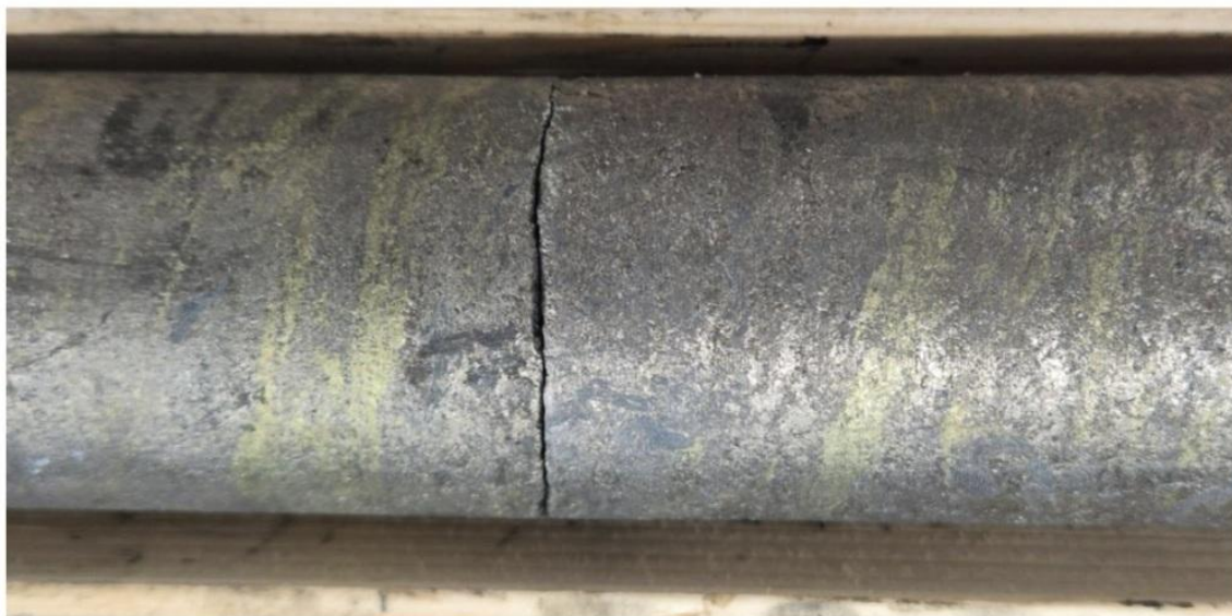
Massive pyrrhotite with about 10% chalcopyrite in regular bands at 85 degrees core angle. Center of photo was taken at 243.75m in drill hole CUP26-06
