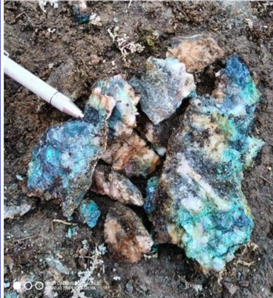
23.90 % Cu, 238.00 g/t Ag, 1.40 g/t Au Digenite, malachite, bornite, calcite vein, cm scale (#C1456119)
