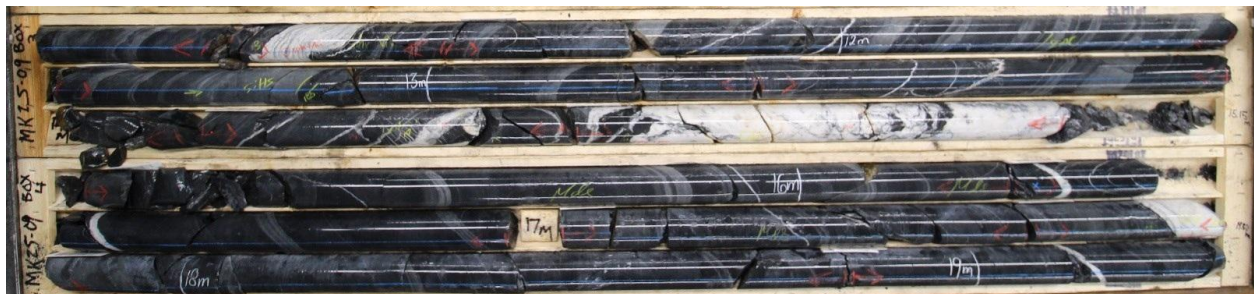
Photograph of drill hole MK25-09 from 12.0 to 19.0 metres (0.65 g/t Au over 9.35 m)
