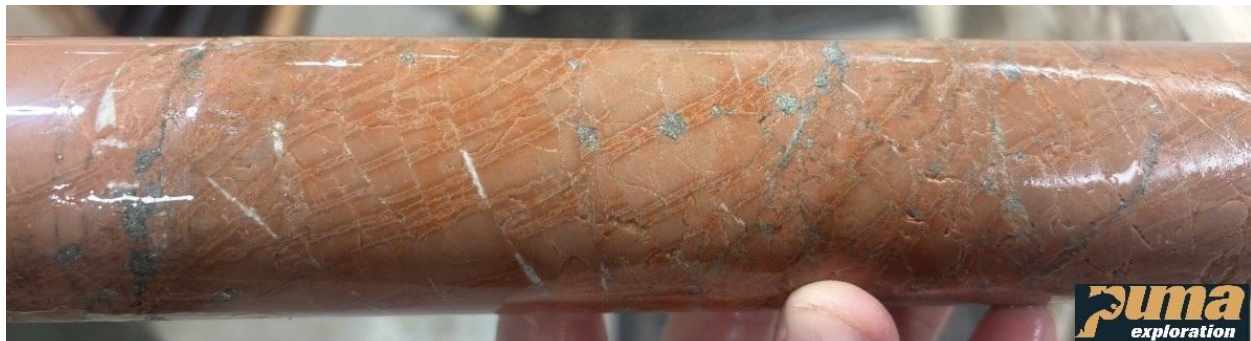
Drill core of typical altered rhyolite intersected in WB26-195
