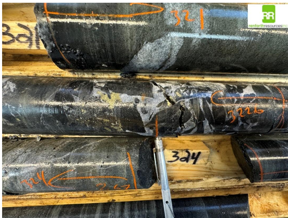
SUR-26-59 - coarse clotty cpy at flow-top breccia in v4 at 322.4-322.6m
