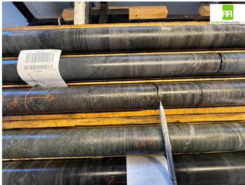
SUR-26-59 - ab-shear with fracture cpy around 284m, calcsil around 285m
